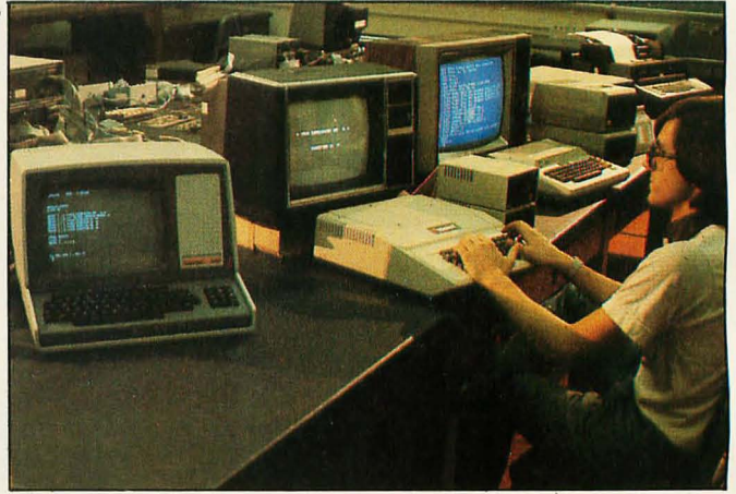
Photo 2: The equipment currently available in the Solo/NET/works laboratory. The terminal at the lower left in Photo 2a is used for the WAG display (as explained in the text). To its right is the IMSAI S-100 computer that emulates the unrooted-tree network and performs the managerial WAG functions. Further to the right are the system console and bus-status monitor; the other microprocessors operate as nodes in the network. Photo 2b shows MATSRCH designer Ivan Zatkovitch using an Apple II computer in a version of the game that requires only one player.
