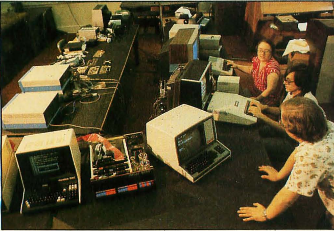
Photo 2: The equipment currently available in the Solo/NET/works laboratory. The terminal at the lower left in Photo 2a is used for the WAG display (as explained in the text). To its right is the IMSAI S-100 computer that emulates the unrooted-tree network and performs the managerial WAG functions. Further to the right are the system console and bus-status monitor; the other microprocessors operate as nodes in the network. Photo 2b shows MATSRCH designer Ivan Zatkovitch using an Apple II computer in a version of the game that requires only one player.
