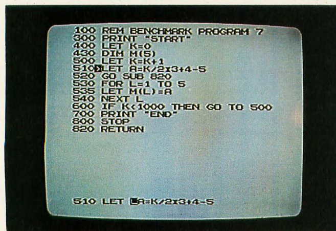
Photo 3: Editing on the ZX80. The cursor (at line 510 at the top of the screen) can be moved via arrow keys to different lines of the program. When the Edit key is pressed, the line being pointed to is copied at the bottom of the screen, where it can be edited. The cursor on the bottom line can be moved right and left; characters can be deleted or inserted at the current cursor position. When the Newline key is pressed, changes made in this line are added to the existing program.
